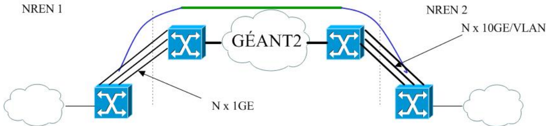
Figure 6.2: Scenario 2 (GE service, accesses via GE & 10GE)
